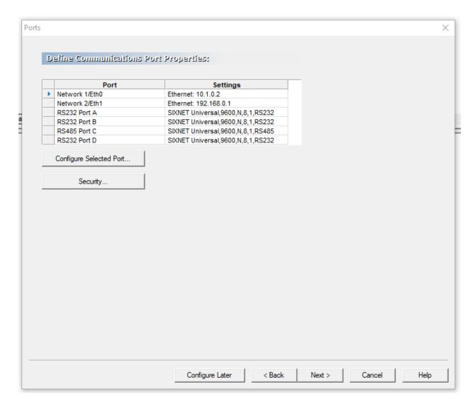
The RTU that has been chosen has 2 separate IP addresses for the hardware.
