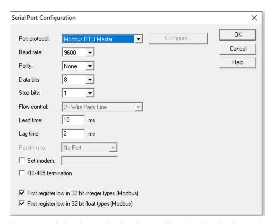
Be sure to set the baud rate, parity, data bits, stop bits, and any lead lag times up based on the device or devices you might be trying to talk too. After you have done this click the OK button
