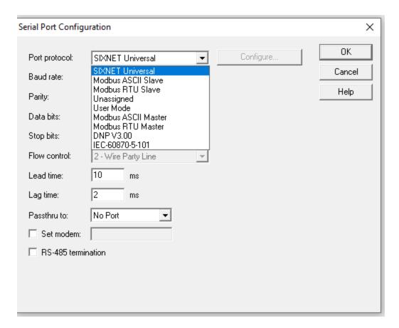
This gives a list of the available drivers that the Serial Ports can be set for. In this case I am going to choose ModbusRTU master, probably our most widely used driver.
