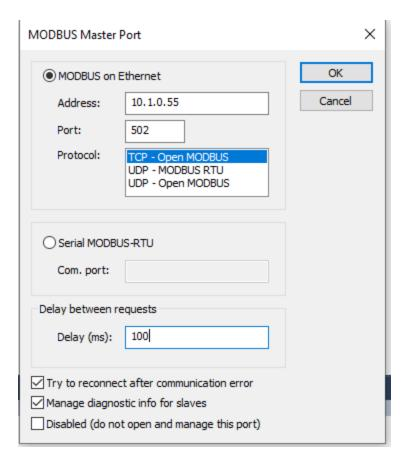
When this box appears, put in the IP address, leave the port at 502 and select TCP-Open Modbus.
