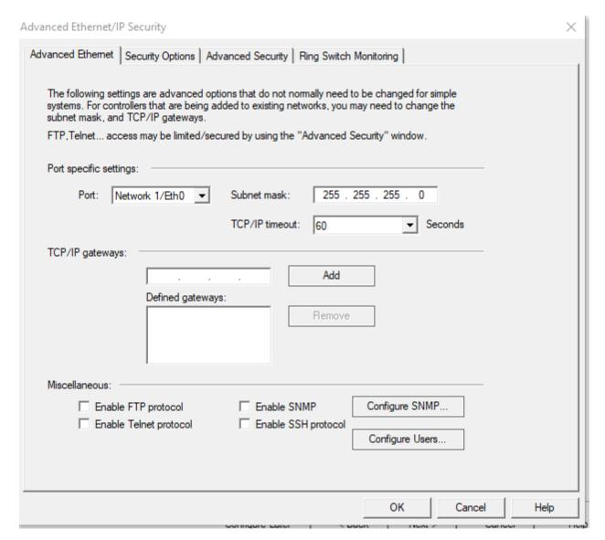
Remember this is simply for Network 1, now we must hit the Port drop down button and select Network 2 and do the same for it.
