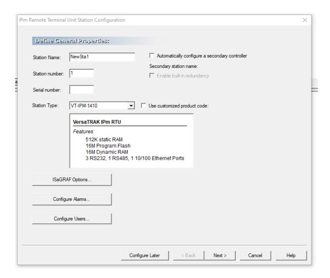
Fill in the Station Name, Station Number, serial number and select the RTU type.
