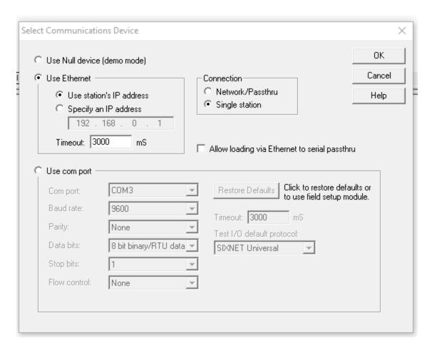
Right now it is set to talk using Ethernet and the stations IP address you set for it. It is a recommended setup to first download thru the serial port B on the unit. So now set up your Communications Device box like below...
