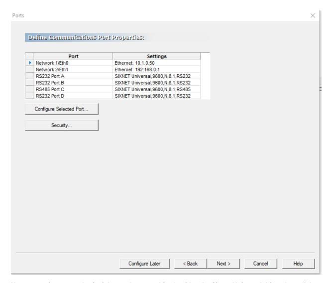
If you are going to use the Serial ports for something besides the Sixnet Universal driver then click on the port letter. The ports are labeled on the front of the unit. I will chose the RS485 port or Port C for this example.
