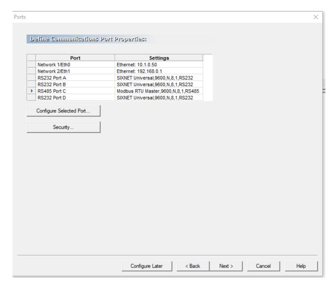
Unless you need to make additional changes to the serial ports you can now download this configuration to the RTU.
